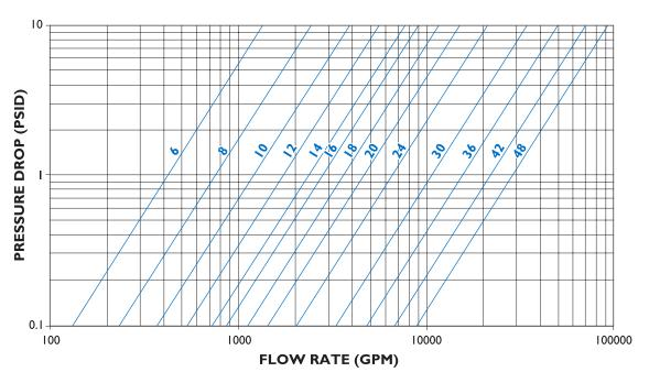
Notes: I. Pressure drop curves are based on water flow with standard screens.
