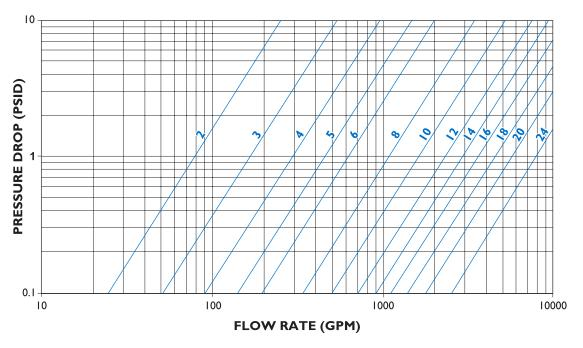
Notes: I. Pressure drop curves are based on water flow with standard screens.
